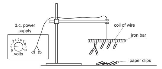
The iron bar attracts steel paper clips when the power supply is switched on.
